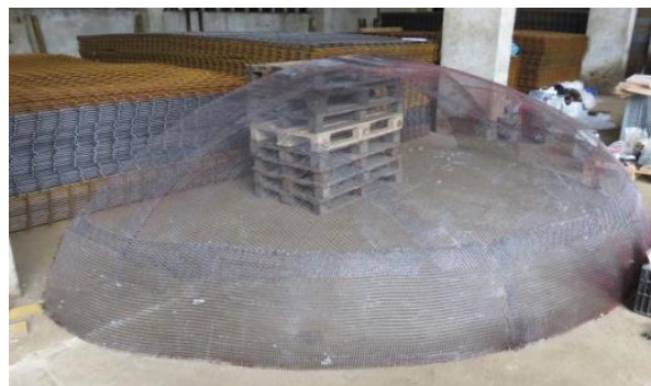
Fig. 2: Filigree reinforcement made of carbon fibers
