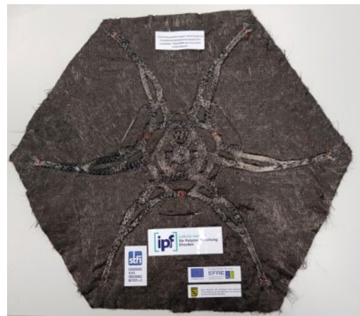
Fig. 4: Lightweight stool on 100 % rCF-nonwoven
